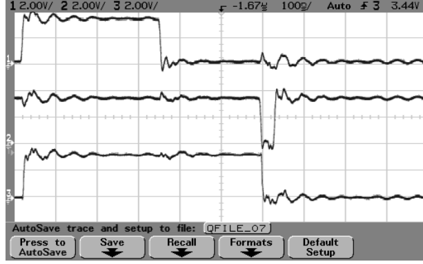
Figure 3.72: Output of the DFT circuitry for the case of R_{open}=\infty , T_{wt}=40\text{ns} . Upper curve: clock signal CK. Middle curve: activation signal \phi . Lower curve: output signal Q.
